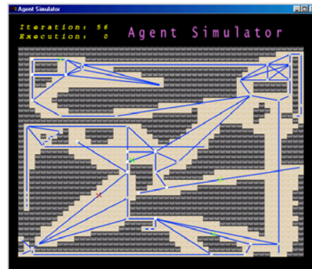
Figure 1 - The map. Black blocks in the maps represent obstacles. The graph of possible paths is shown. The graph has 87 edges and 62 nodes. This figure is also a snapshot of the simulator.
